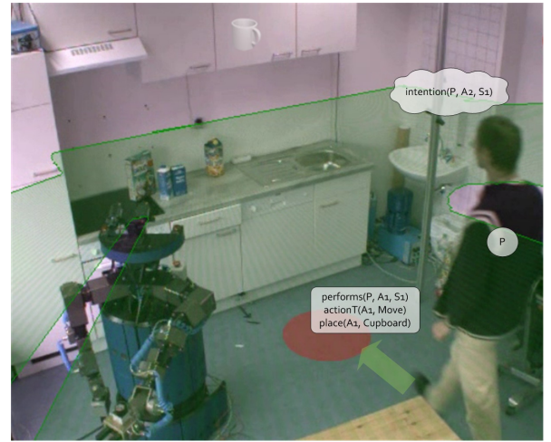
Fig. 7. Recognizing human intentions allows the robot to react, i.e. either to support the human or to keep clear. Action-related concepts like the places where one stands when performing an action can help the robot decide what a human is currently doing.
