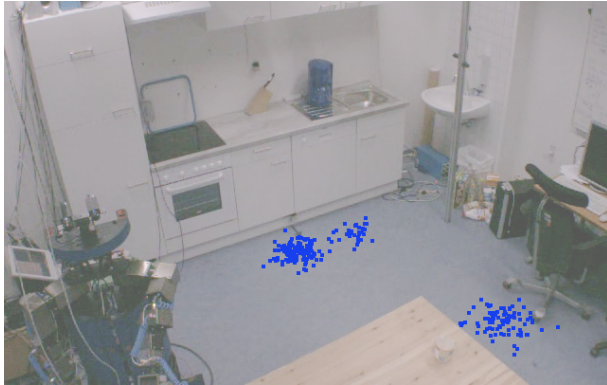
Fig. 4. Raw positions of manipulation actions (dark blue dots), recorded while the robot (bottom left) set the table in our demo kitchen. Due to the noisy measurements, it is hard to find a link between actions and positions.
